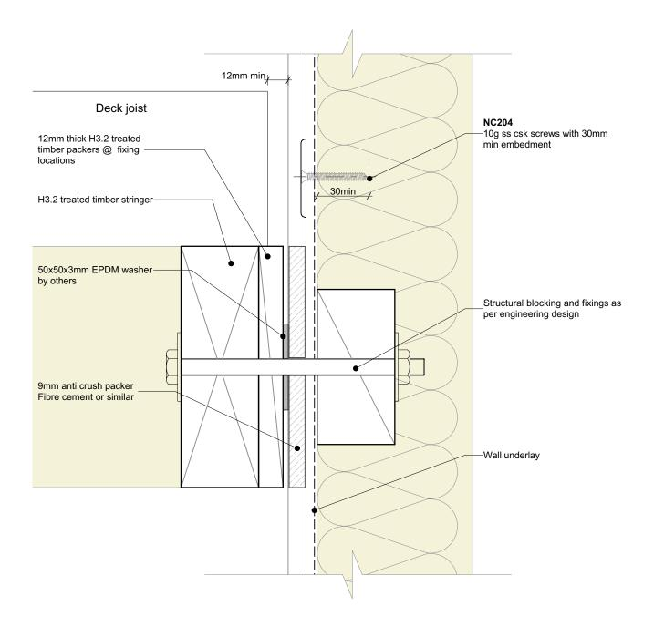
• Nu-Wall is a hollow profile and requires packers to prevent crushing under presure
