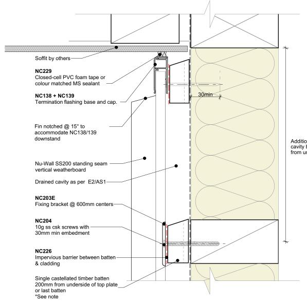
Additional nog and castellated cavity batten to be 200mm max from underside of top plate
