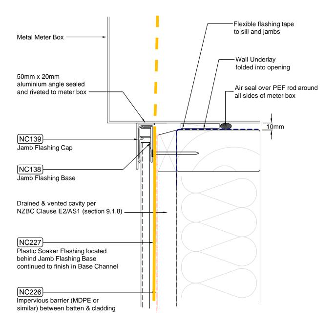
NW-V015C - Vertical Cladding over Drained & Vented Cavity - Meter Box Sill Detail Scale 1:2
